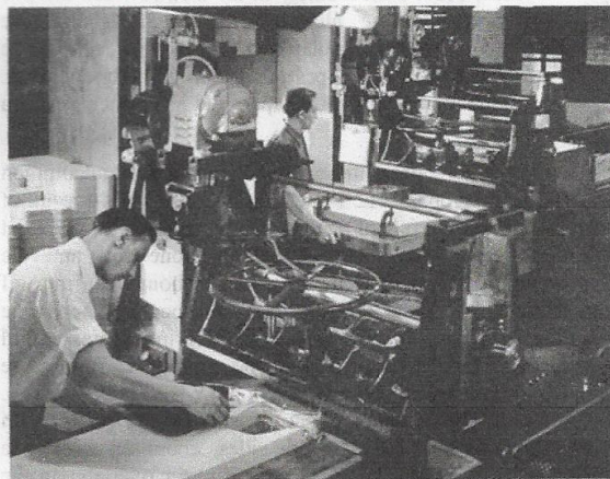
Figure 4. Typical envelope cutting knife form (die) with cutting edge on bottom, top flap of envelope at lower rear. Below, a man is laying the knife die on a pile of sheets which will be moved forward into the hydraulic press to force the knife through the pile of sheets cutting the blanks.
